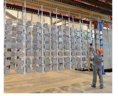
The plant is equipped with an automated horizontal powder coating line (Wurster, Germany) for aluminium and steel parts. Main production line parameters:
