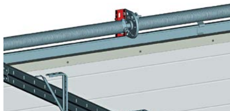
Intermediate bracket (IB-4508) Lagerblech (IB-4508) Patte-support intermédiaire (IB-4508)
